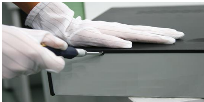
Figure 2. 1 Remove the Cover
